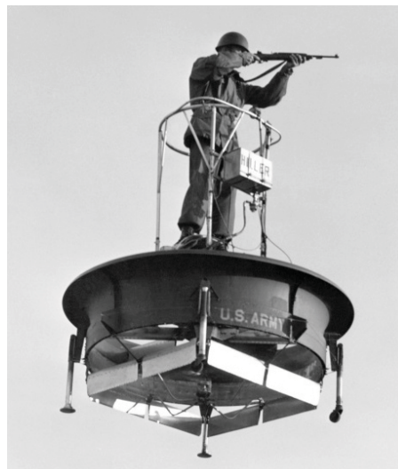
Ühe mehe lennualus (nn Hiller Flying Platform ), 1957, US armee tellimus-eksperiment. Foto: The Flying Platforms & Jeeps
